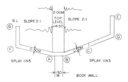
The height of abutment above foundation concrete = 14.50 - 9.60 = 4.90m. The bottom width required is about  $4.90 \times 0.4 = 1.96$  or say 2.00m The section indicated in figure.
